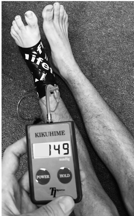
Figure 2 – The Kikuhime pressure monitoring device applied under the floss band.
