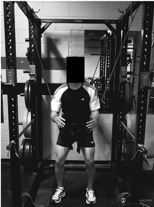
**Figure 1.** Example of the assisted jump setup. A harness and elastic bands were attached to the participant and to the squat cage above.
